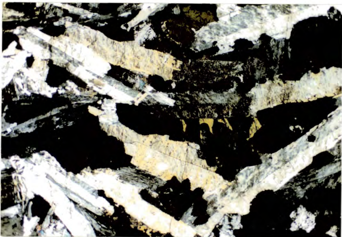
Plate 3.1. G232. \times 11 . XPL. Typical laminated syenite from the Upper Series. Tabular, perthitic alkali feldspars define the lamination, with aegirine-augite (just above and to the left of centre), and nepheline (mainly altered to brown giesseckite). Interstitial cancrinite (with yellow interference colours) can be seen in the centre of the field of view.
