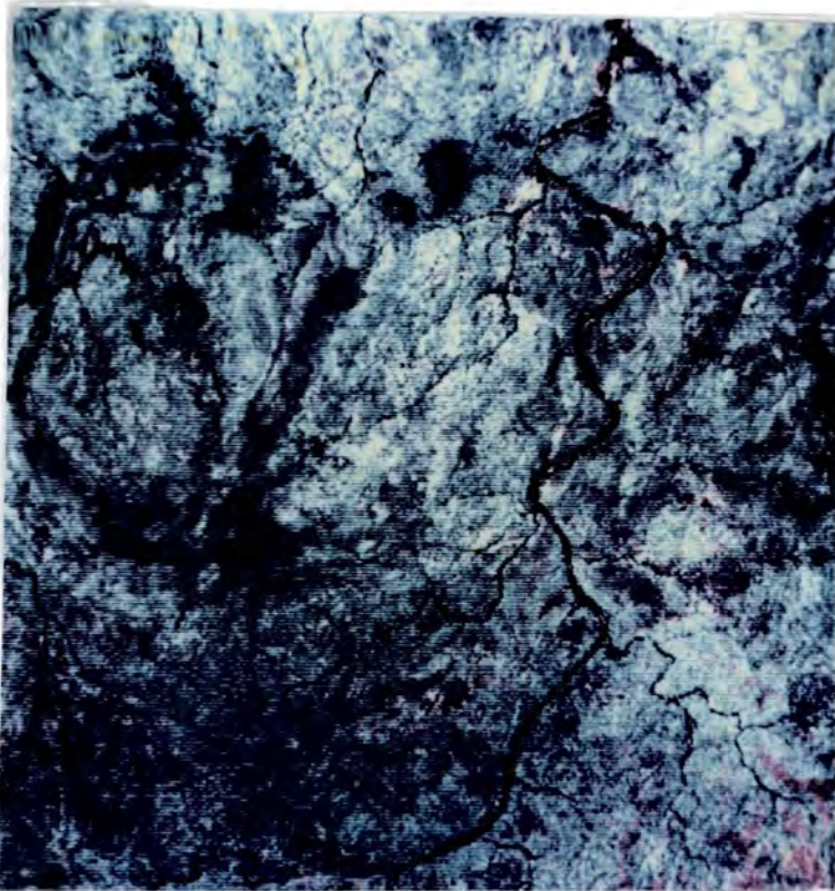
Plate 3.2 Colour Composite of the 10.7\mu\text{m} , 9.2\mu\text{m} and 8.4\mu\text{m} Raw TIMS Channels Displayed as Red, Green and Blue respectively, Camp Oven Test Site.
