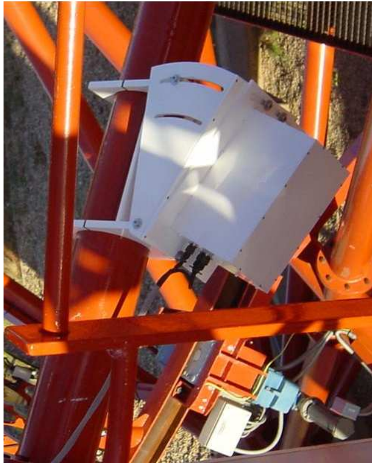
Figure 3.6: KT 19 radiometer paraxially mounted in one of the four H.E.S.S. telescopes.
