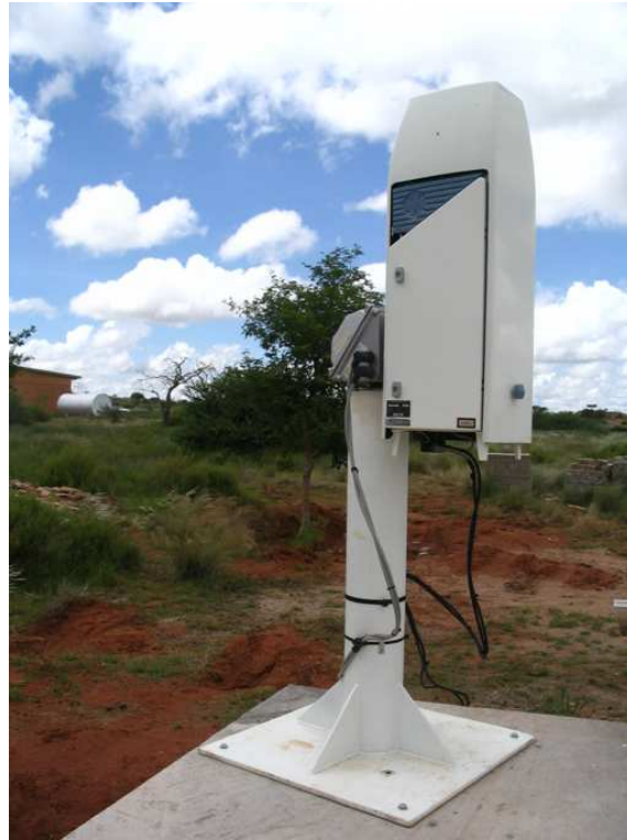
Figure 4.1: CT25K Vaisala LIDAR installed at the H.E.S.S. site in Namibia.
