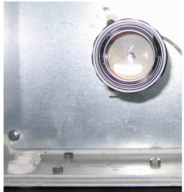
Figure 5.9: The camera equipped with the big lens ( f = 105 mm) in its separate box.
