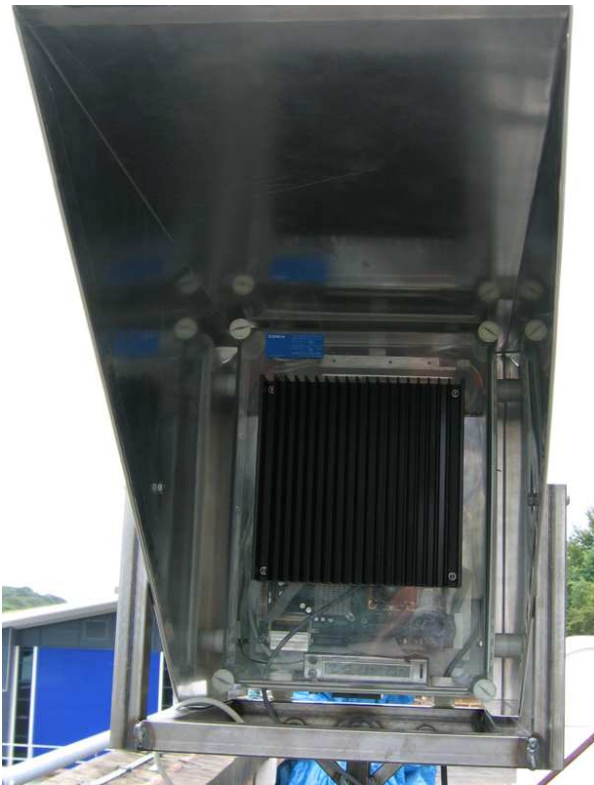
Figure 5.8: The light receiver with the lid closed. The heat sink was used in the initial stages of development. The CMOS camera, located at the bottom right of this photograph, was later relocated to a separate box to maintain temperature stability.
