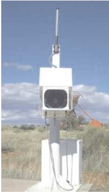
Figure 3.13: Light receiver with the lid open. Taken from Le Gallou (2005).
