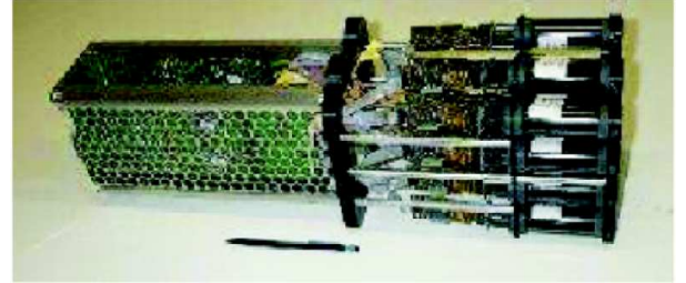
Figure 2.25: A drawer containing 16 PMTs and the associated electronics. Courtesy of the H.E.S.S. Collaboration.
