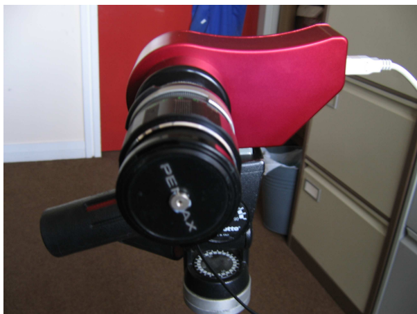
Figure 6.2: The new ATIK-16 CCD camera equipped with a 135 mm lens.
