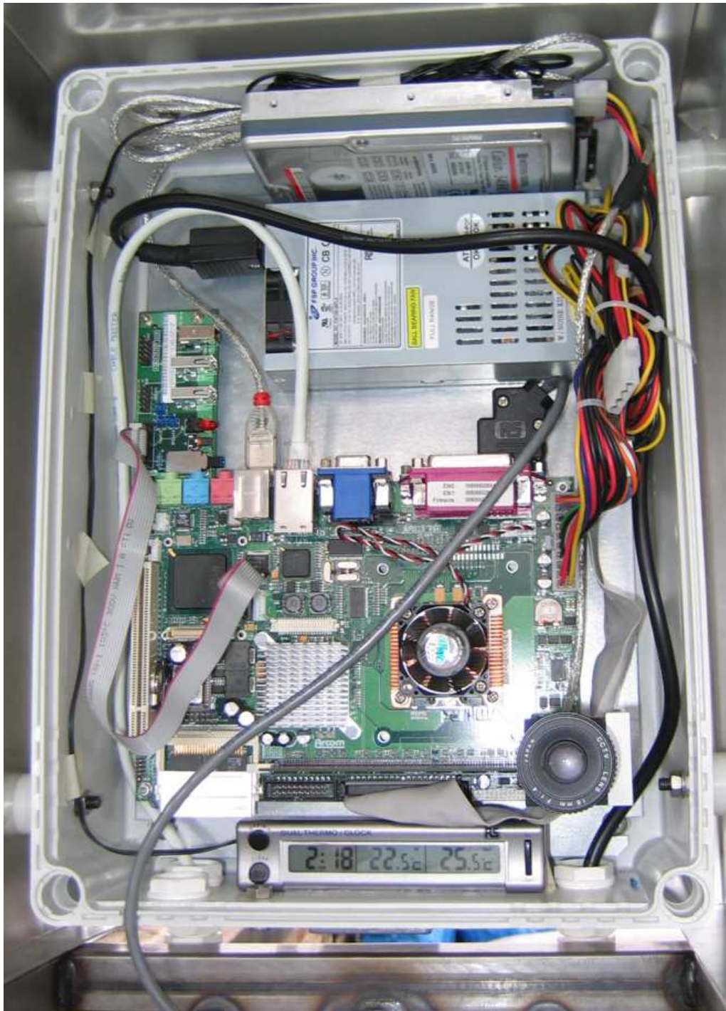
Figure 5.7: The light receiver. One can clearly identify the Apollo SBC with its power supply and hard disc, the camera equipped with the 16 mm lens and a simple temperature monitoring device.
