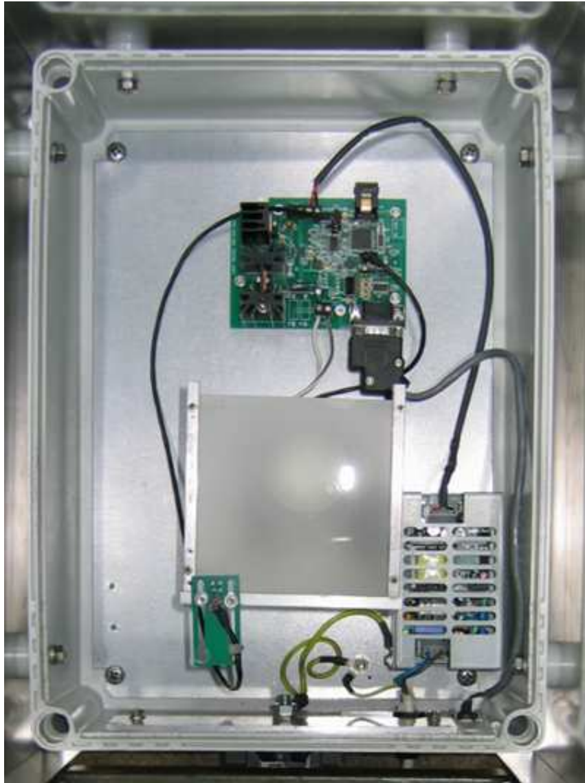
Figure 5.4: The light transmitter. The controller system is towards the top of the enclosure and the power supply is at the bottom right. The LED is located behind the large, square diffuser.
