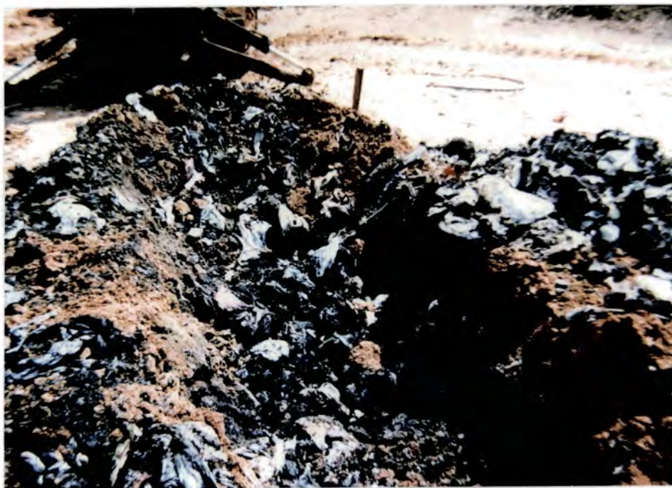
Fig. 1.6 A close-up of GDB landfill cover with the soil partially removed. The remain of waste, after embedded for about 10 yr, is mainly plastics, with the organics degraded. The cover was dug for lying water pipes and cables.
