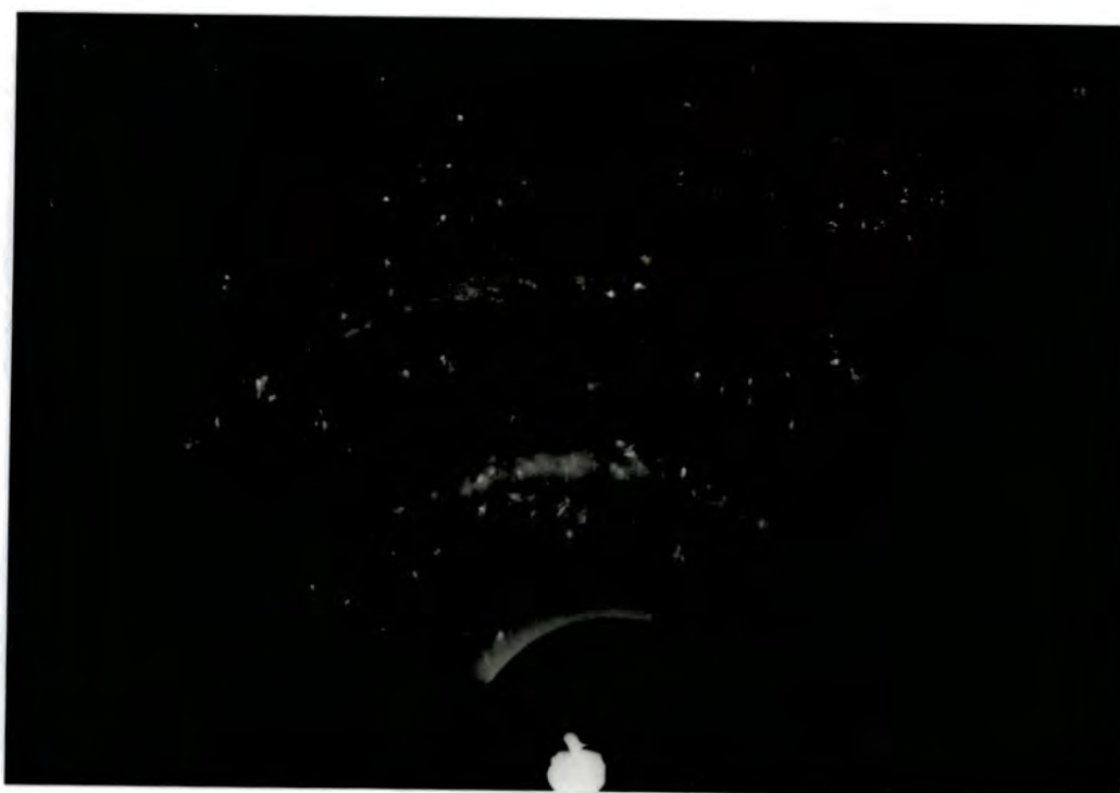
FIG 4.9: A typical RHEED pattern for black alumina
