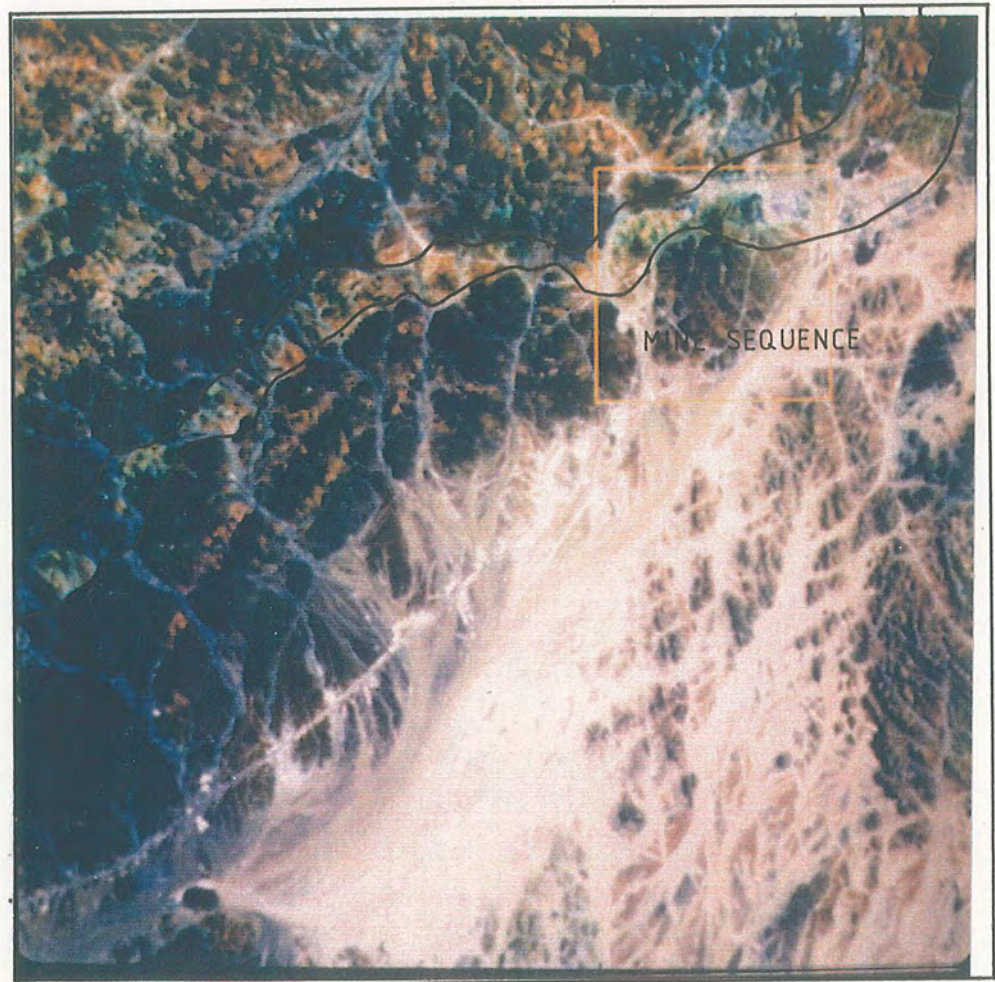
Fig. 6.15 False colour composite of Mahd Adh Dhahab deposit; TM data, band 7,5, 2 in red, green and blue respectively. The hydrothermal alteration appears in greenish-blue colour (inside the yellow sequence), the boundary of the mine sequence can be followed easily.
