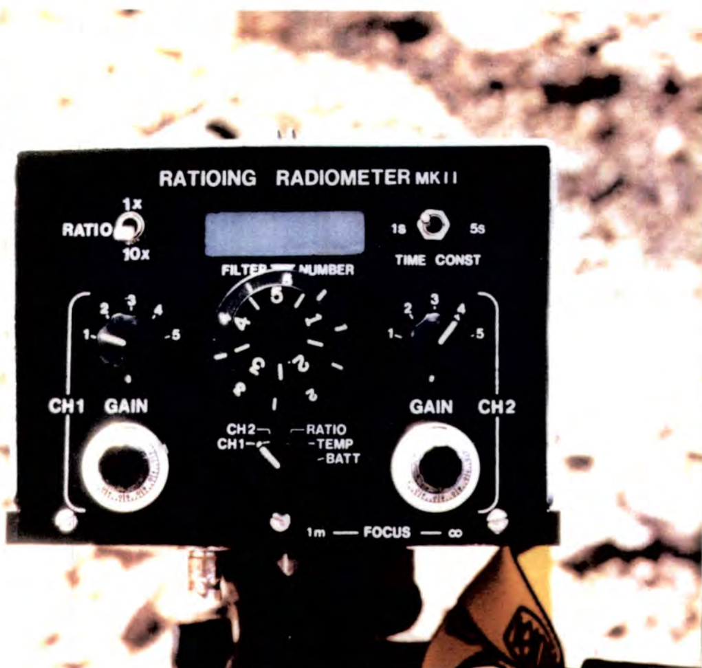
Fig. 3.28 The back of the Barringer HHRR showing the display panel and detector controls.
