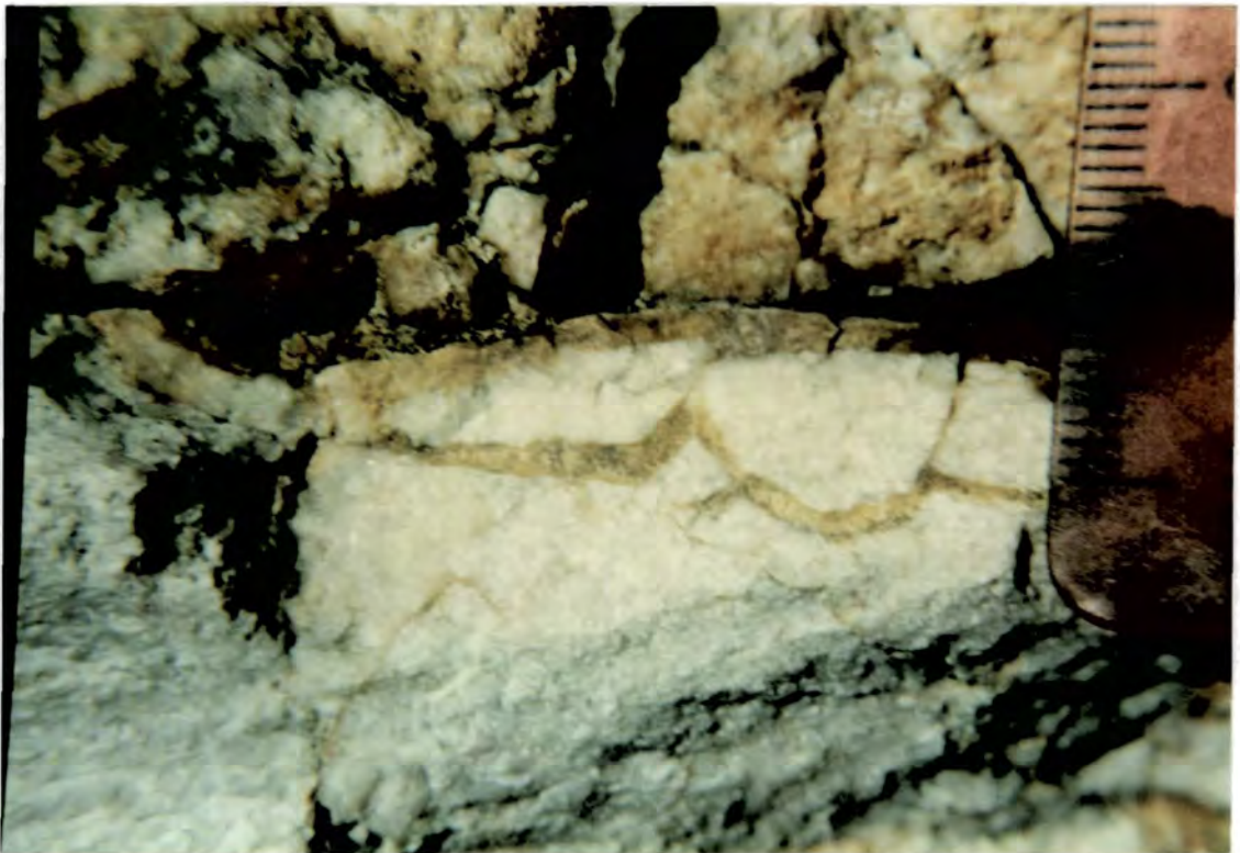
Figure 4.2 Fracture associated with the breccia zones filled with a combination of smectite and montmorillonite (See Section 4.2).
