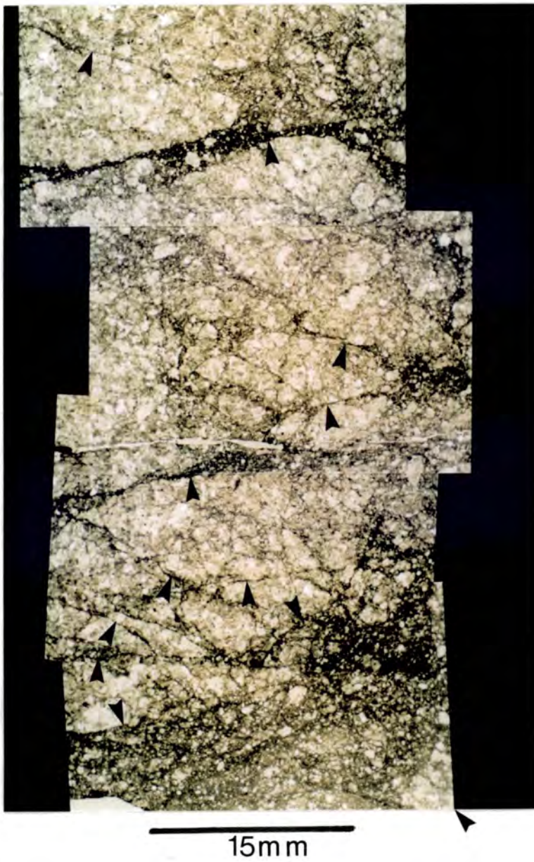
Figure 4.11 Photomicrograph of sample 8i (see Section 4.3.3.6). Field of view is 15mm. The main fuge zones are arrowed.
