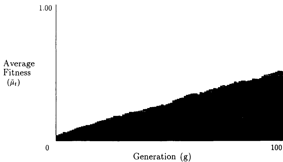
Graph C.18 The change in performance obtained using a population of 175 with a subsampling factor of 2.
