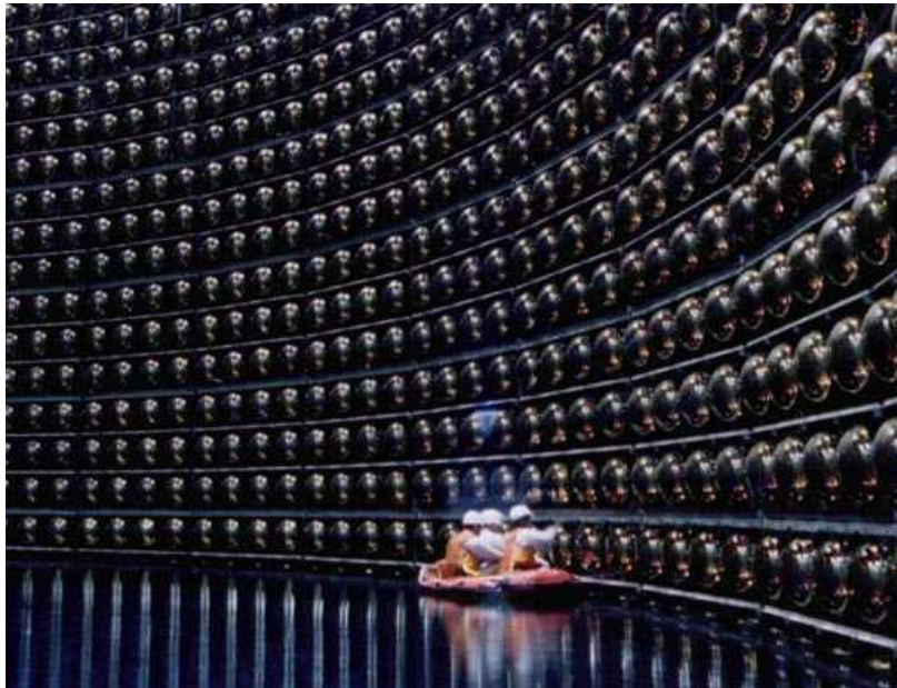
Figure 3.2.: The 50 kton water Čerenkov detector, Super-Kamiokande.
