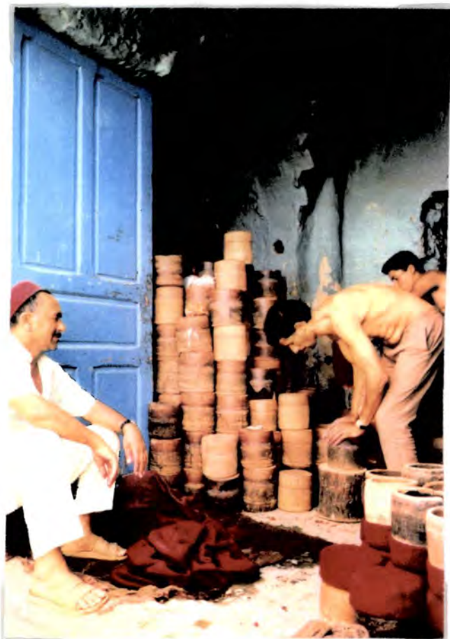
6(a) Newly dyed chéchias are placed on pot moulds before going into a special drying cabinet. Workshop near Dar Lasram, north-central Medina
