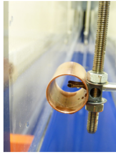
(a) Kiel-reverse probe, detail of the pressure intake and the positioning bar. Due to the pressure taps are protected by the outer cylinder, the positioning bar has little influence in the flow streams.
