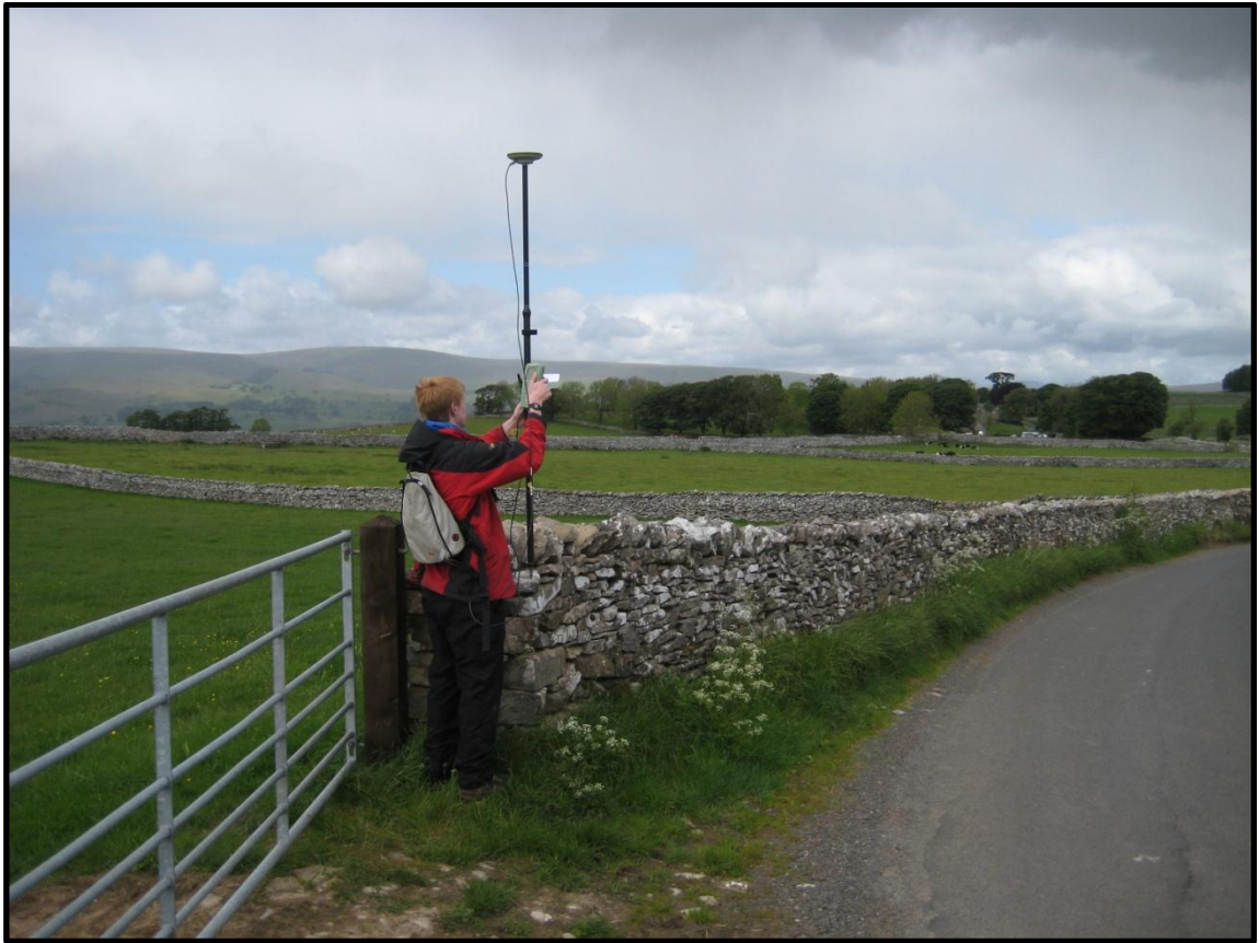
Figure 9: Ground control was collected with a differential GPS with accuracy >0.025 m. Due to the high resolution of the imagery, individual rocks were easily distinguishable and so these were used as control points during the survey.
