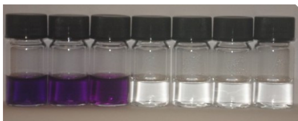
Figure 4.8 Degassed 1.0 \times 10^{-4} mol dm -3 solutions of host 132 in MeCN in the presence of one equivalent TBA salts of the following anions (from left to right): succinate, malonate, acetate, chloride, bromide, nitrate, perrhenate
