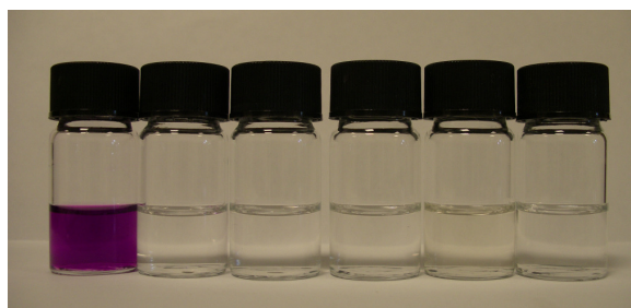
Figure 4.9 Degassed 1.0 \times 10^{-4} mol dm -3 solutions of hosts 134 in MeCN in the presence of one equivalent TBA salts of the following anions (from left to right): acetate, malonate, chloride, bromide, iodide, nitrate
