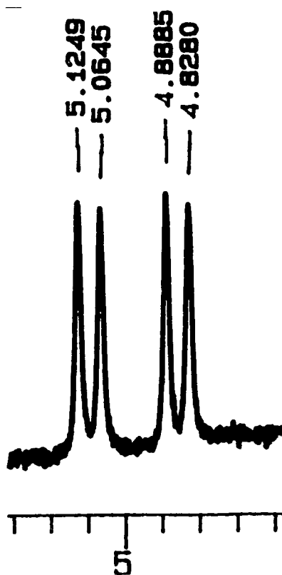
Figure 54. ^1\text{H} NMR of (±)-methyl 2-fluorophenylacetate (192) in the presence of [\text{Eu}(\text{tfc})_3]
