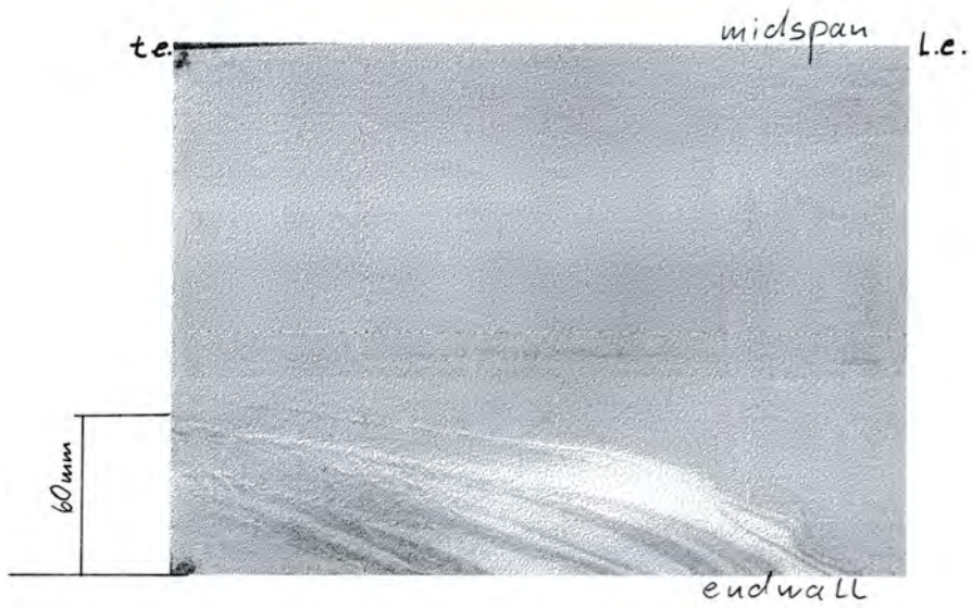
Figure 4.35: Flow Visualization at Suction Side: Low Angle - 250%
