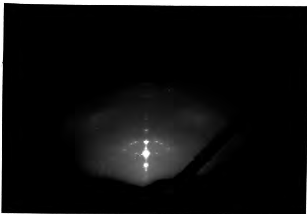
Figure 5.36 RHEED pattern for 6 layers of perylene:TA 1:12.
