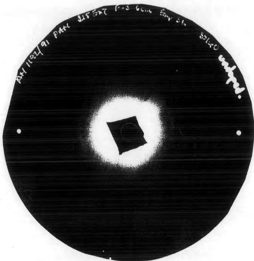
Figure 6.14 Flat-film X-ray photograph of an 230% elongated EB film with the stretch direction vertical. The two circular diffraction signals seen in Figure 6.13 are now observed as arcs along the equator.
