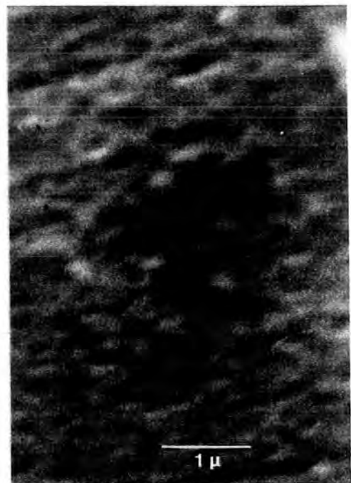
Figure 7.9. Crater formation on copper electrodes, with a 50 nm oxide layer.
