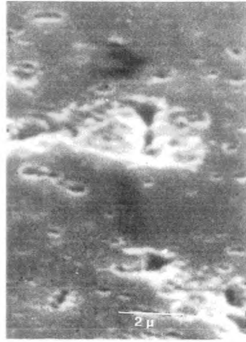
Figure 6.16. Crater formation on copper electrodes. Aerodynamically driven with an arc velocity 8 ms -1 .
