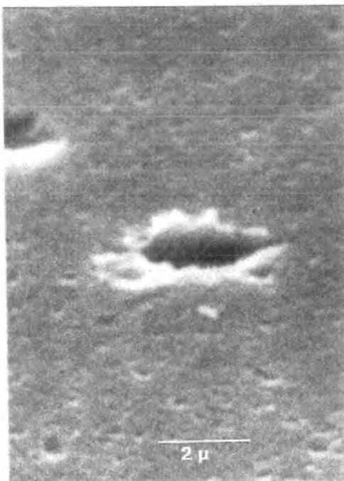
Figure 6.3. Crater formation on copper electrodes. Magnetically driven with an arc velocity 70 \text{ ms}^{-1} .
