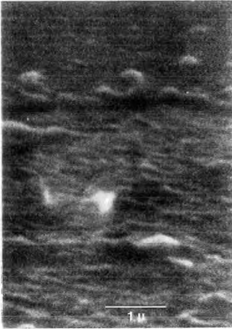
Figure 7.2. Crater formation on copper electrodes, with a 100 nm oxide layer.
