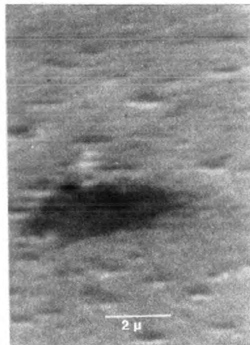
Figure 6.4. Crater formation on copper electrodes. Magnetically driven with an arc velocity 80 \text{ ms}^{-1} .
