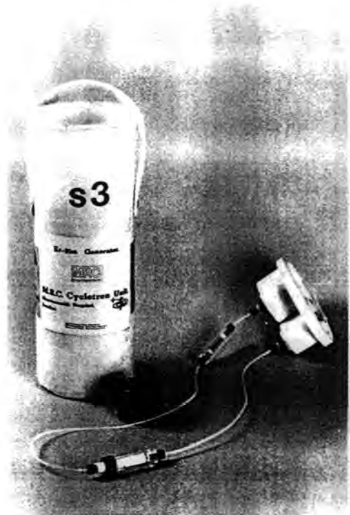
Fig. 1-2B. The MRC ^{81}\text{Kr}^m solution generator for use with an isotonic dextrose eluant. Shown with the zirconium phosphate column (white) out of the lead shield and the series rubidium trap column.
