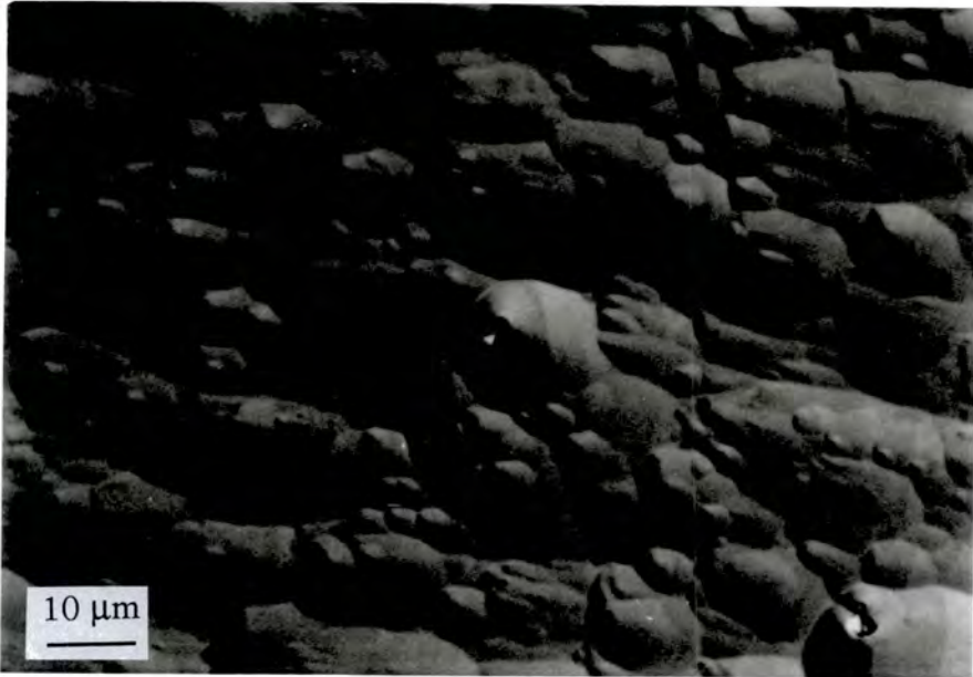
Figure 3.7c Surface morphology of a 24.5 μm thick (001)CdTe/GaAs epilayer.
