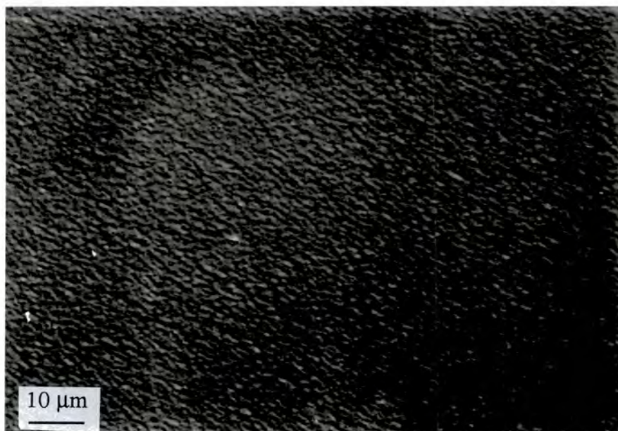
Figure 3.7a Surface morphology of a 0.60 μm thick (001)CdTe/GaAs epilayer.
