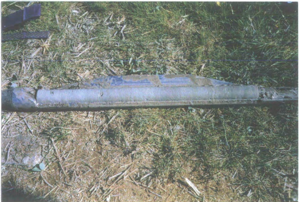
Plate 2. Russian corer with 300 cm-350 cm core section from Amarador in place (22/3/95, 16:00).
