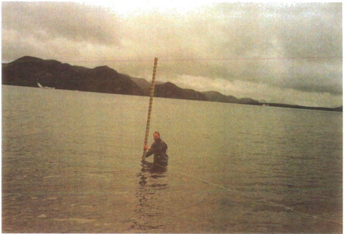
Figure 4.5: Measuring the height of a (submerged) strand line relative to the lake level.
