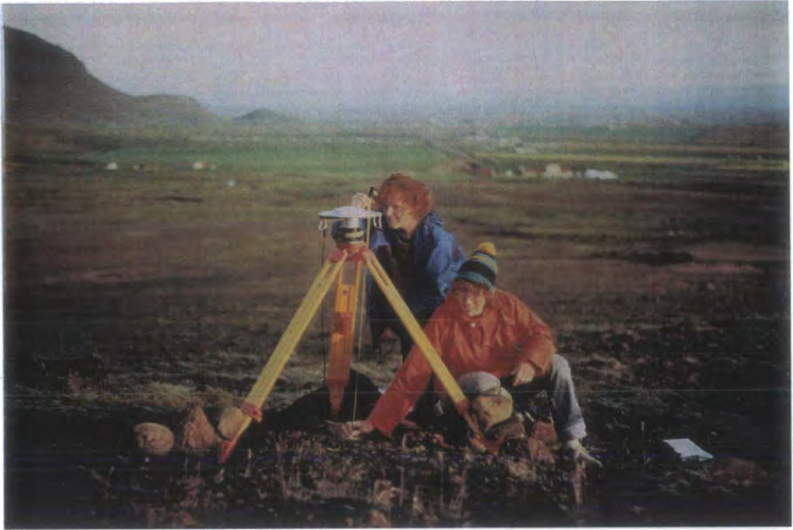
Figure 4.1: A typical set of GPS field equipment.
