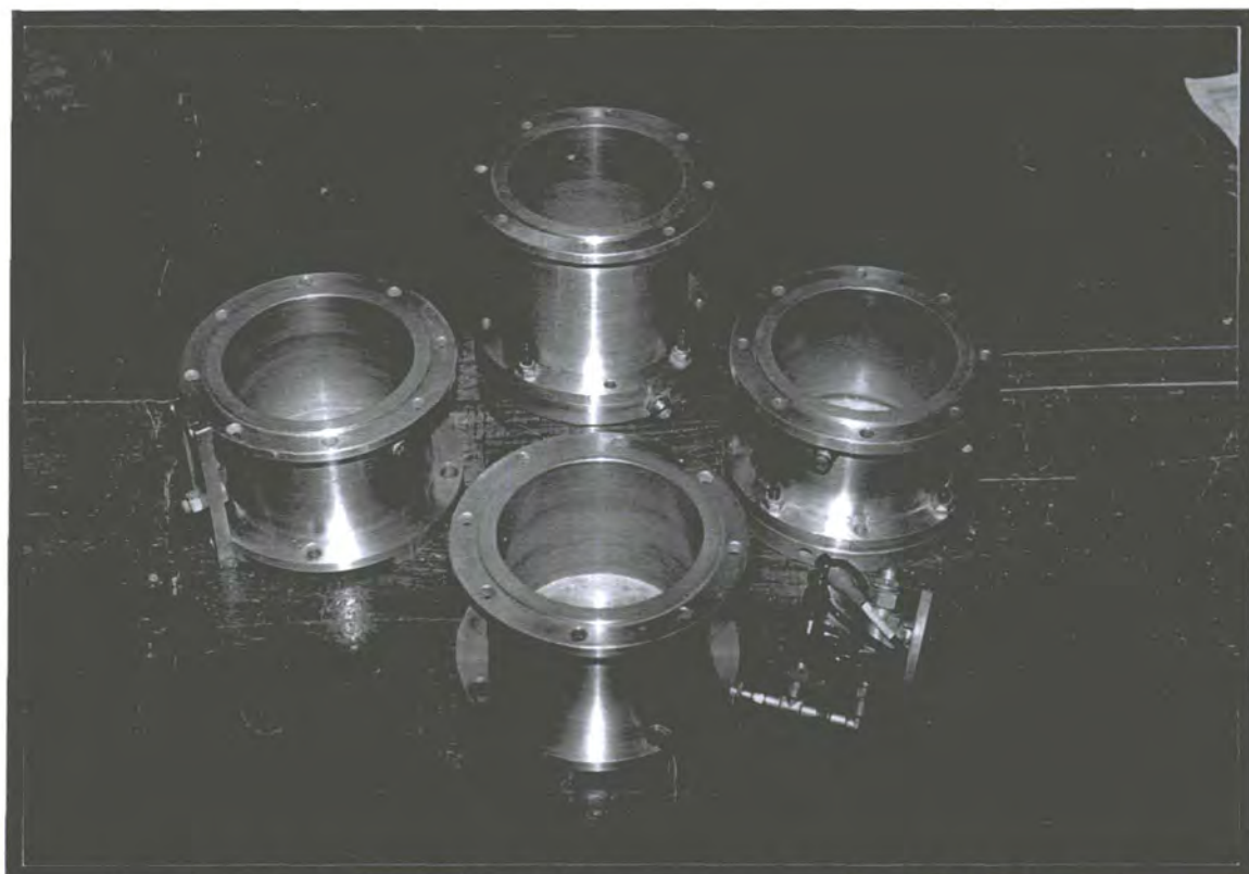
Plate 4.3. Available cell bodies (clockwise from the top: modified tall cell; modified cell; modified cell with integral base; cell adapted for horizontal vibration).
