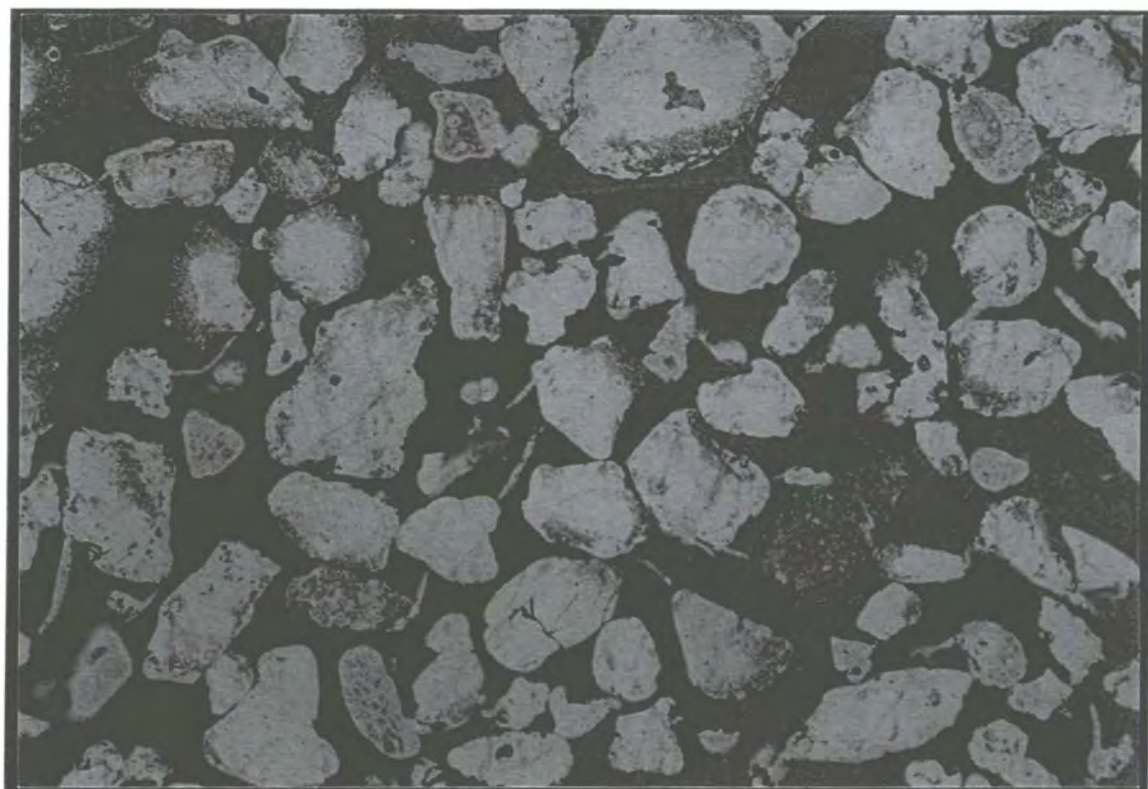
Plate 4.10. Thin-section of medium Leighton Buzzard sand (x 25 magnification).
