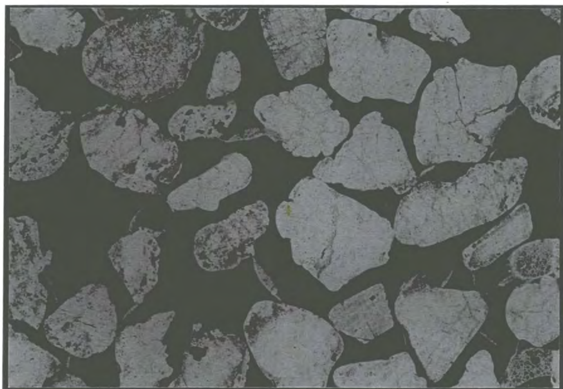
Plate 4.11. Thin-section of coarse Leighton Buzzard sand (x 25 magnification).
