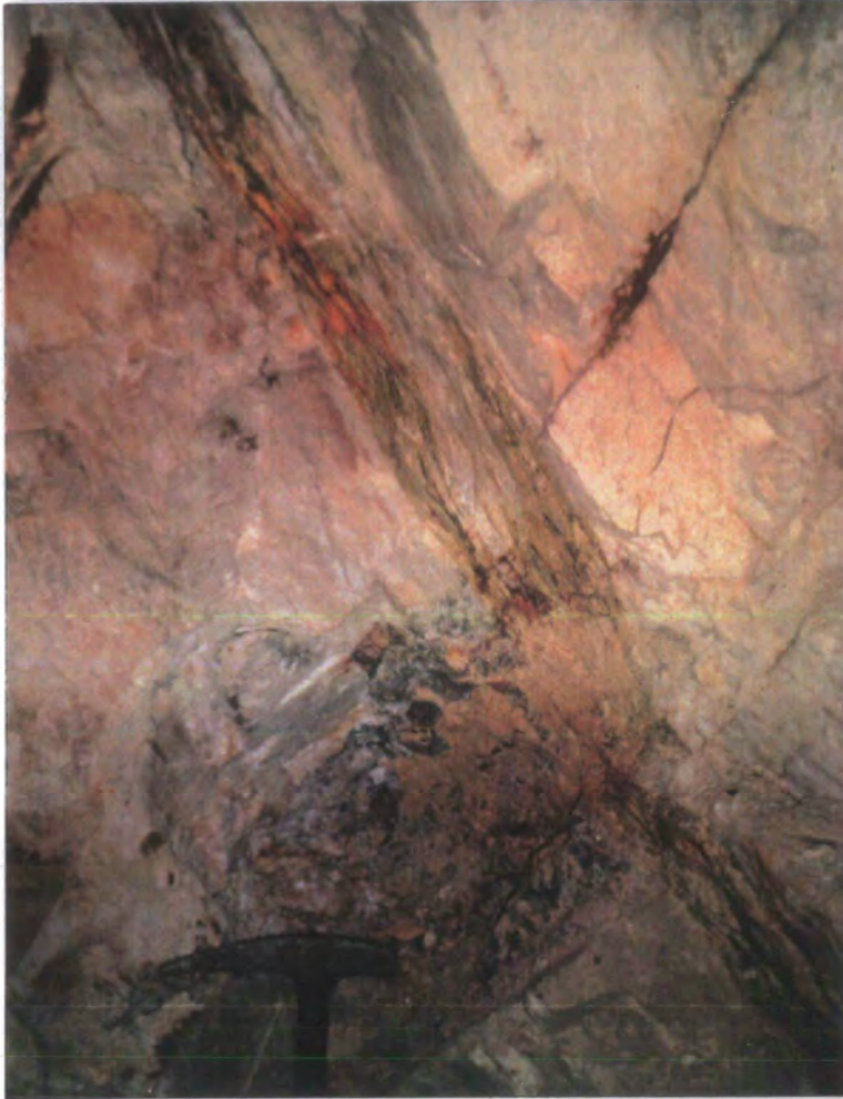
Photo 5.2.4- Ductile shear zone, parallel to bedding, observed in a small gallery close to the lake, in the Amethyst Mine.
