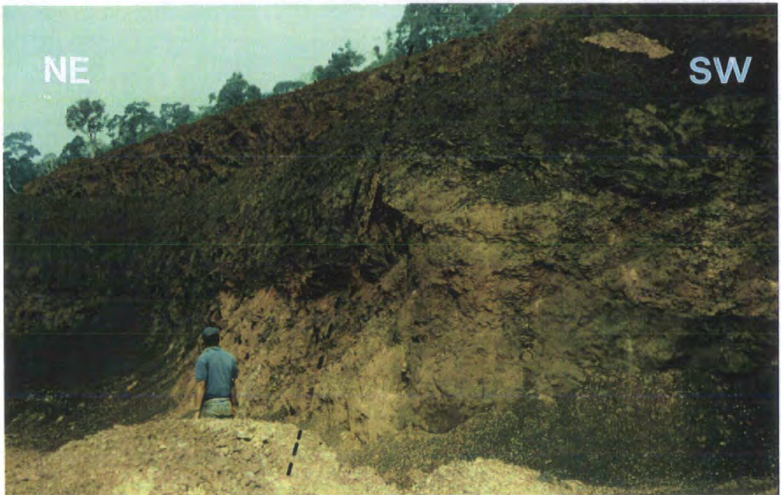
Photo 4.2.8- E-W normal fault with dip-slip displacement of about 2m affecting the contact between Mn-rich mudstones and red siltstones, on top (approx. coordinates: 1150E-000).
