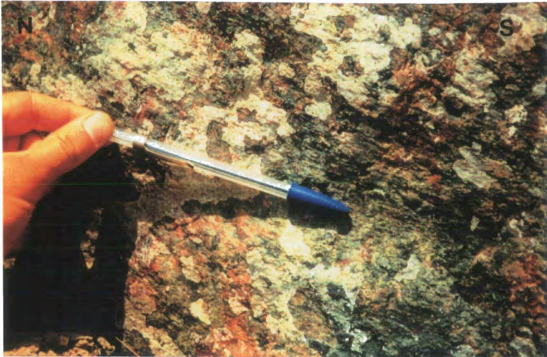
Photo 6.6- Low-angle slickenlines indicating predominant strike-slip displacement along later N-S fractures planes in the Central Carajás Granite.
