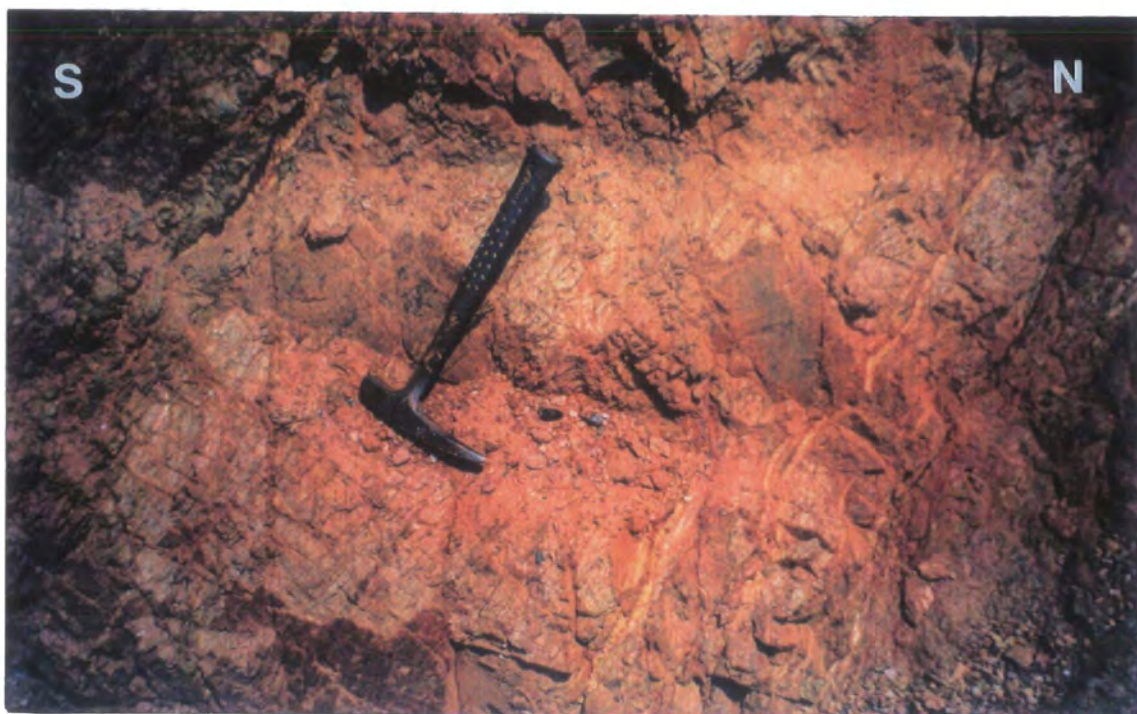
Photo 5.3.6- Typical rock exposure in the Cutia Mine. A slaty cleavage is overprinted by a sub-parallel disjunctive anastomosing cleavage and cut by orthogonal sets of fractures.
