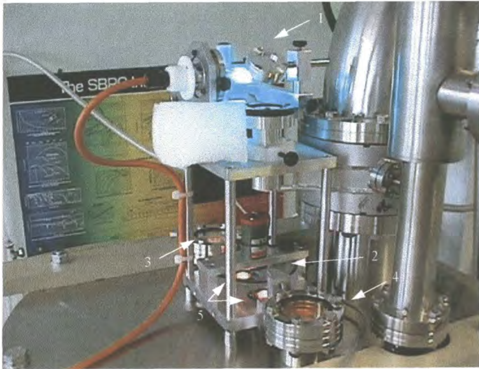
Figure 6. Photograph of the HC cadmium lamp and optics (1) and mechanical chopper (2) used for vapour pressure monitoring through the optical windows (5). The viewing ports (3) and (4) allow direct observation of the source and crystal respectively.
