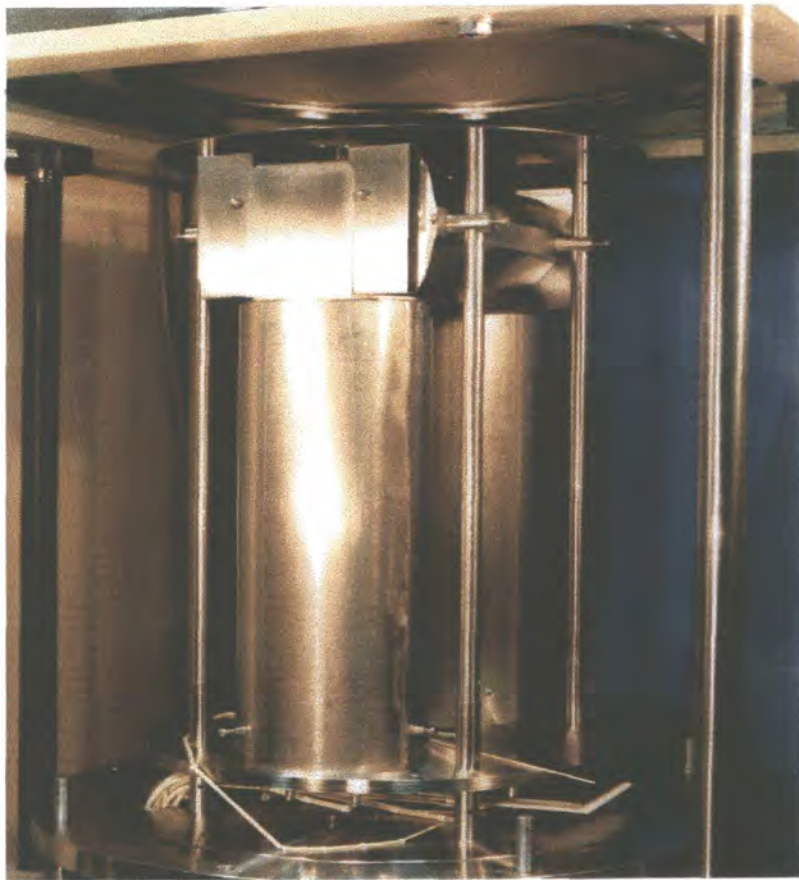
Figure 4. Photograph of the growth system of figure 3 after all the heat shields have been put in place. Three of the four stainless steel rods that support the QHL's and the molybdenum heat shields elements are visible.
