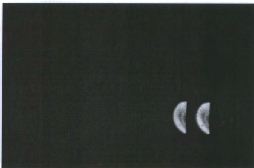
Figure 10-5 Unfocused image of Jupiter with half wave plate @ 45 deg
