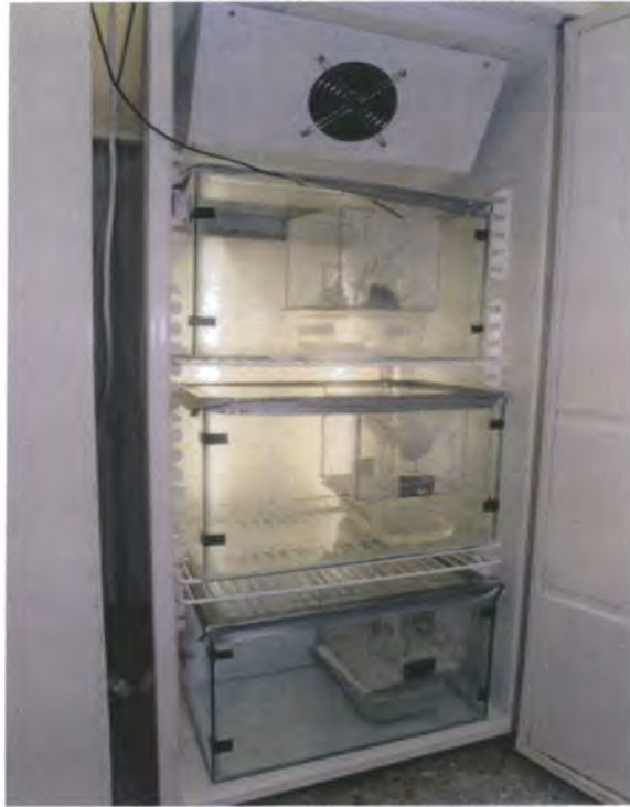
Plate 6. Set up for adult An. gambiae s.s. studies in environmental chambers inside growth chambers.
