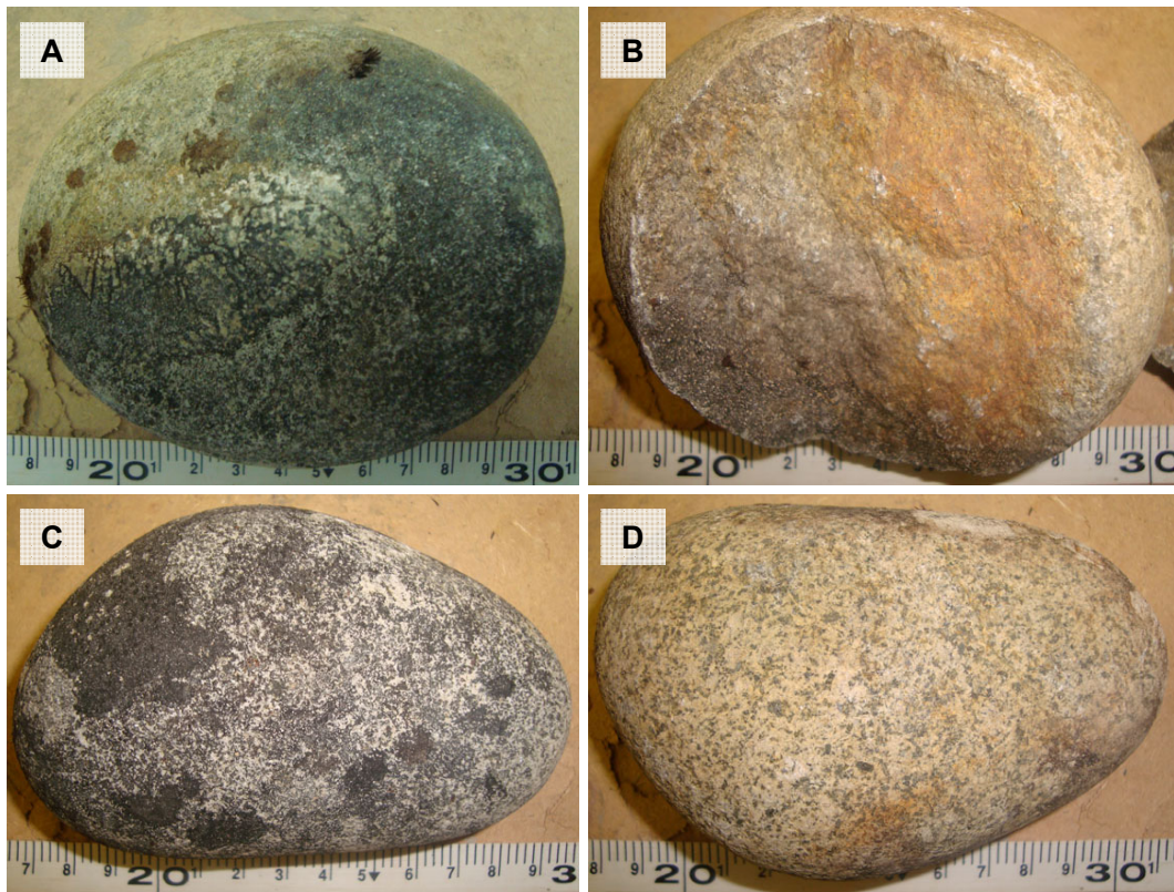
Fig. 7.4 Clasts sampled from Noel Hill for cosmogenic exposure age dating, (a) showing the difference in the surface of the exposed and buried parts of the clast; (b) inside of clast; (c) upper exposed surface of clast; (d) lower buried surface of clast
