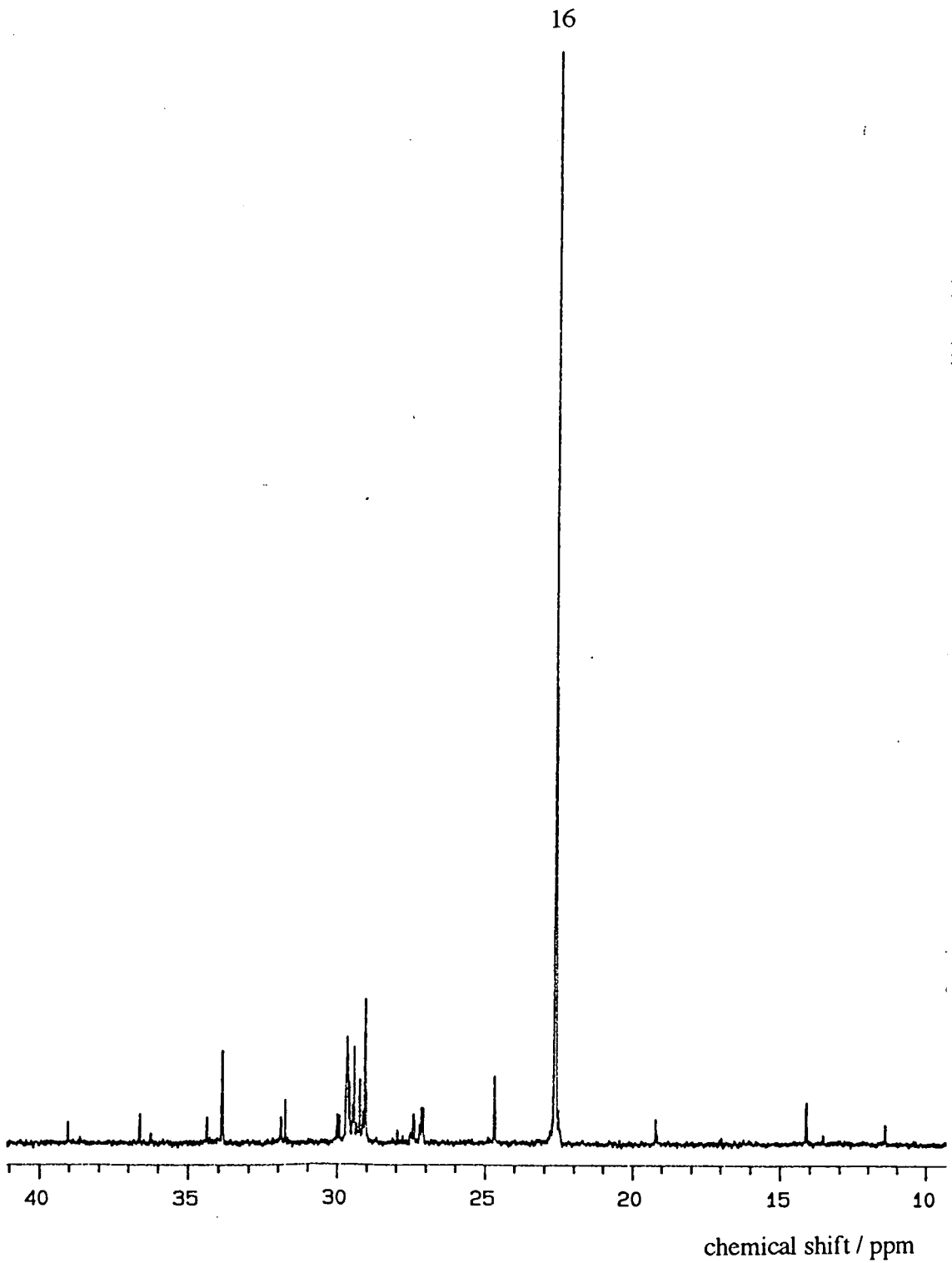
Figure 5-14 Section of the ^{13}\text{C} NMR of the fatty acid extract from S. cinnamomensis fed with sodium [3-^{13}\text{C}] -(R,S)-isobutyrate
