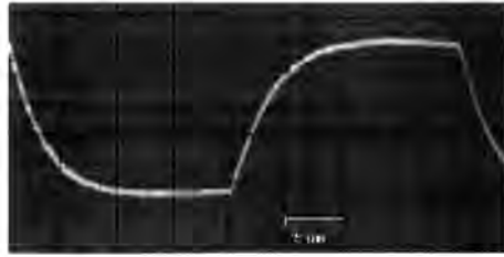
Figure 3.3: Response of the mirror to a 25Hz input signal. One horizontal graduation represents 5ms.
