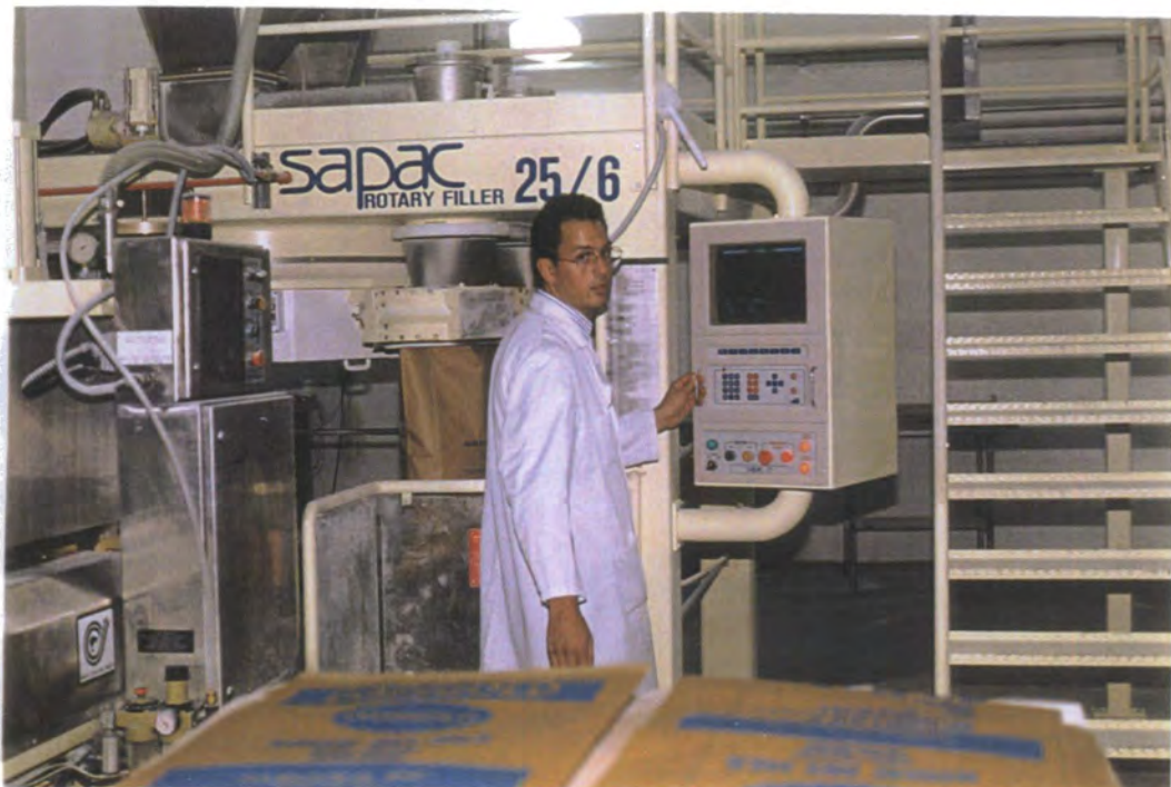
Photo 2: One operator fills eight 25 kg. skimmed milk powder (SMP) bags per minute with the Sapac (NZ) rotary filler, at the Darigold farmers' cooperative plant in Lynden, Washington, USA (all photos).
