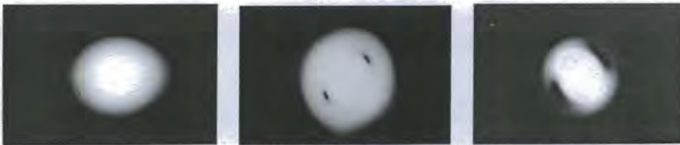
Figure 3.6. Left: An overexposed image of the standard end beam profile. The profile is quite clearly elliptical, with an ellipticity of approximately 0.6. Centre: The beam profile from the taper end. The image was overexposed in an attempt to bring in the cladding modes, which do not appear. Right: The same profile seen through a polarisation analyser. The axis of the analyser is horizontal (across the image).
