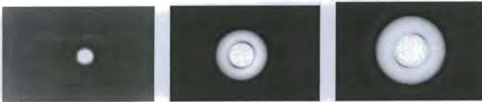
Figure 3.5. Left: The output profile of the standard ( f/6 ) end. Centre: An overexposed image of the tapered ( f/18 ) end's beam profile. The first diffraction ring from the cladding modes is clearly evident. Right: The same profile with a longer exposure time. The second diffraction ring is just visible.
