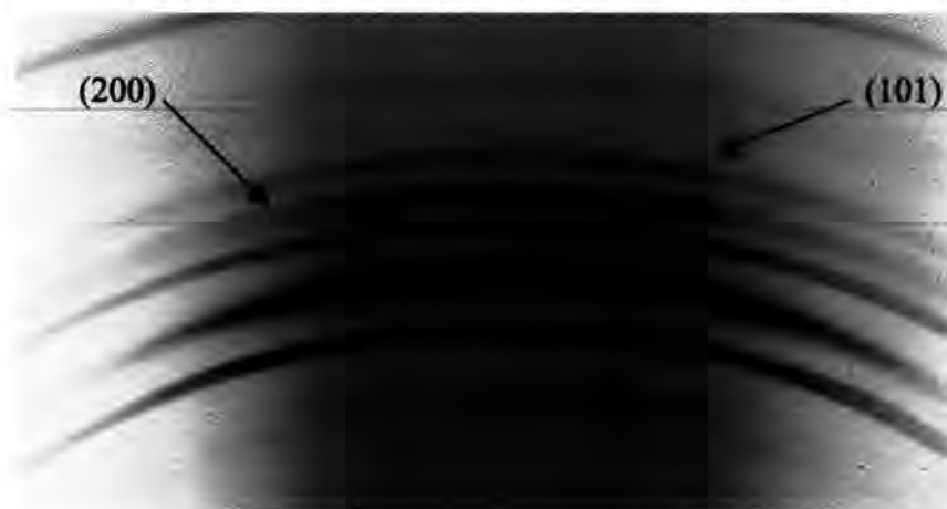
Fig. 6.7: CCD camera image of the diffraction rings in sample Sn3 . The strong diffraction rings not labelled are from the sample holder.
