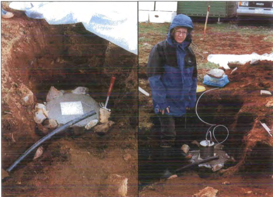
Figure 3.6 (Left) Seismometer pit after initial preparation, showing base of concrete poured onto bedrock, surrounded by boulders and with a ceramic tile mounted as a flat base for the sensor. The black drainage pipe prevents the pit from flooding. (Right) Guralp CMG-40T seismometer positioned on ceramic tile in base of pit.
