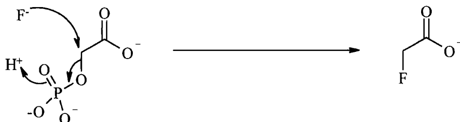
Fig. 1.24: Nucleophilic substitution of a phosphate group by fluoride.
