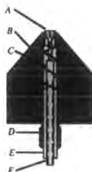
Figure 3.11.2.2 – A schematic diagram of the goniometer head construction. The key is: A: collet B: copper body C: spring D: 1/4 in UNF E: spring tension adjust F: release button. The figure has been reprinted from reference 8.
