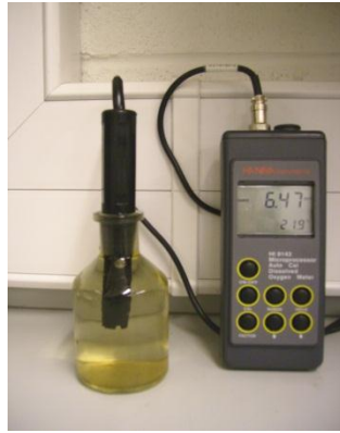
FIG. 3.2: Use of dissolved oxygen meter during a BOD experiment
