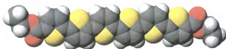
Figure 4.2.12 Molecular model for a sexithiophene derivative \alpha,\omega -di-substituted with two ethyl ester groups. The distance from one ether oxygen to the other is ca. 26 Å.
