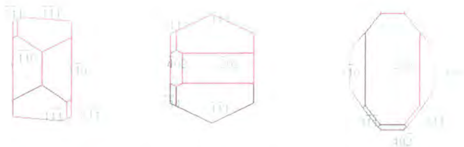
Fig. 4.1. Three perpendicular views of the crystal morphology predicted for dl-aspartic acid by BFDH method.
