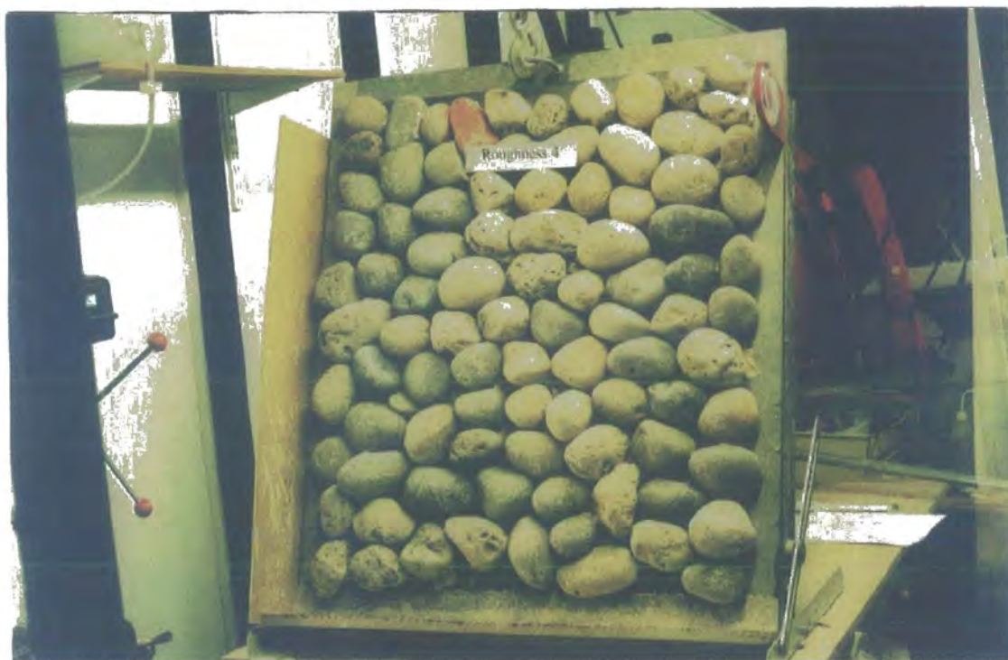
Figure 3.11 One of the artificially-made bed roughness plates. The example shows a tilted metal base plate on which natural coarse gravels (b axes in 64-96 mm size range) were secured.
