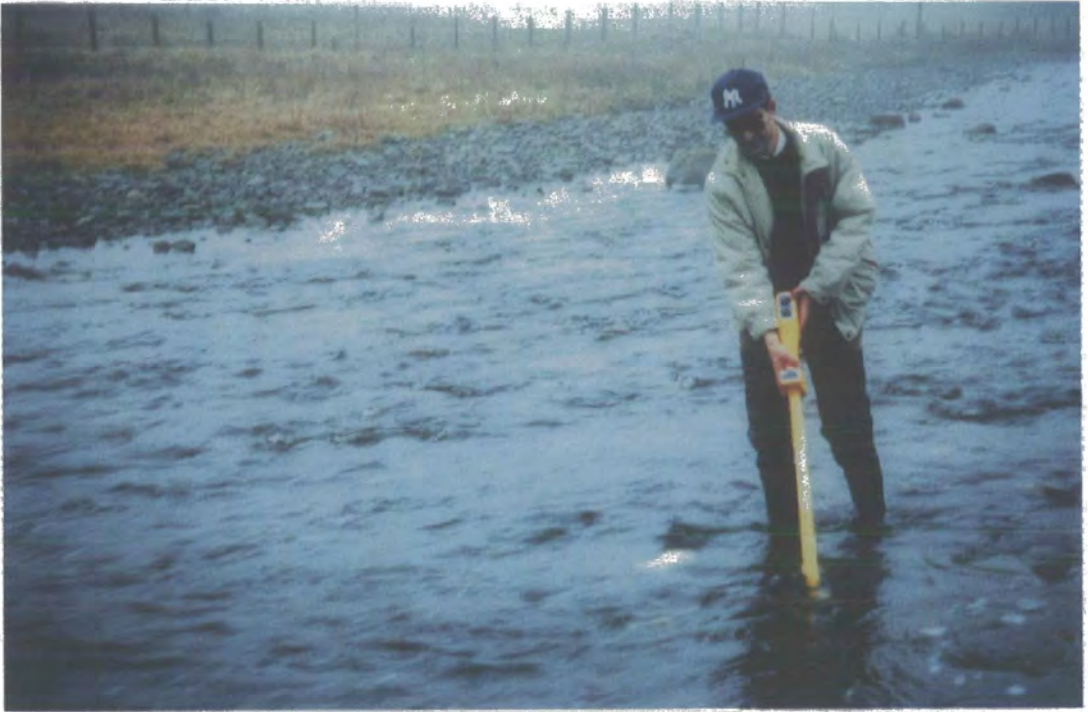
Figure 3.8 Searching for magnetic tracers at the Upper Tees Site. A magnetic locator was used during all searches.
