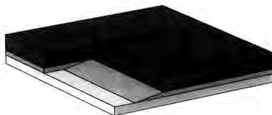
Figure 5.4: Schematic diagram of a bevelled thin film bi-layer on a glass substrate
