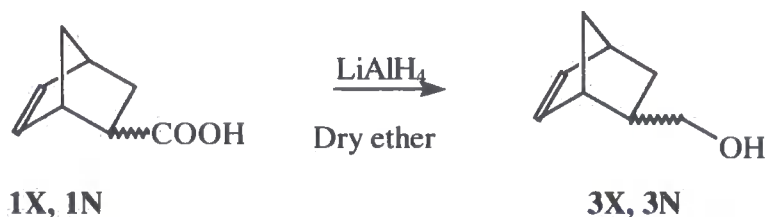
Figure 2-6: A schematic diagram of the synthesis of bicyclo[2.2.1]hept-2-ene-5-methanol.
