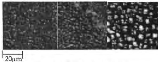
Figure 4-11 MORPIP, D2 and D16 doped PDLCs (from left), observed under the cross polarised microscopes.
