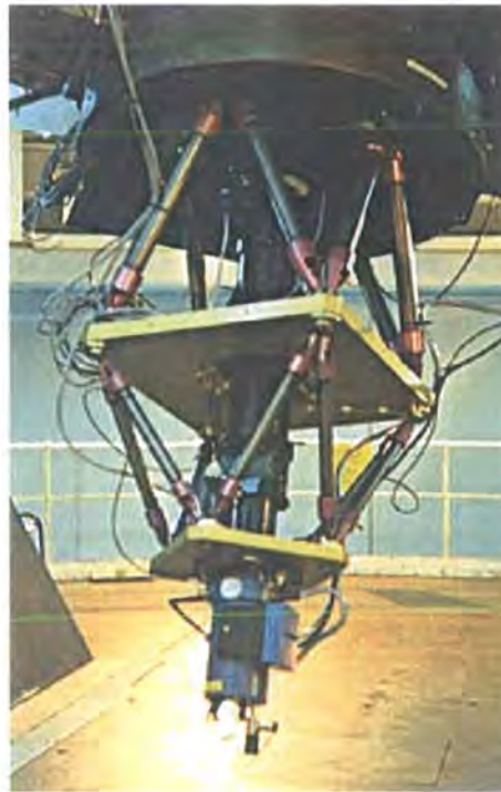
Figure 4.1: Photograph of the SAURON IFU mounted at the Cassegrain focus of the WHT.
