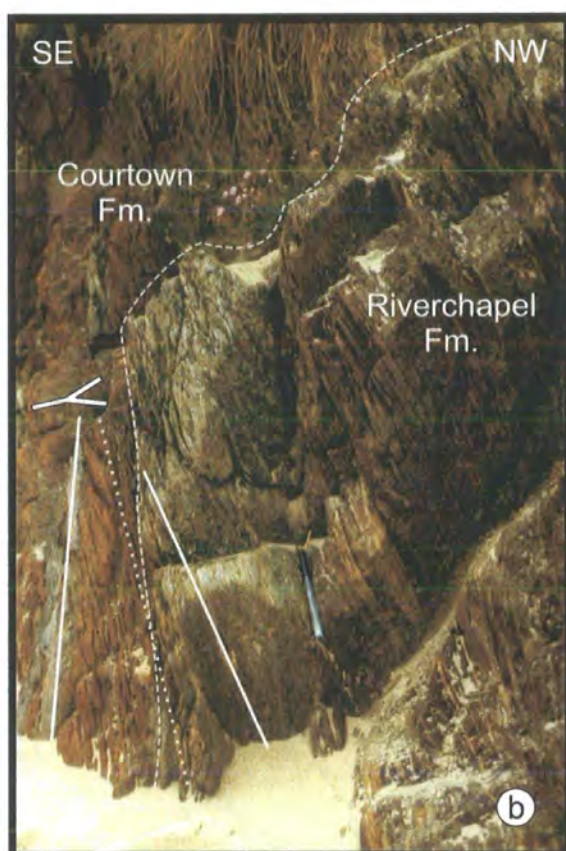
Plate 4.5. (a) Riverchapel Formation north of the shipwreck (Fig. 4.10, grid ref. 22056125). The bedding is folded by sinistral kink folds (scale on lens cap is 5cm) (b) The angular unconformity between the Courtown Fm. (Duncannon Grp.) and the underlying Riverchapel Fm. (Ribband Grp.). The unconformity is irregular with several 10's cm of relief (dashed line) in-filled by sediments of the Courtown Fm. The bedding (solid lines) in the Riverchapel Fm. dips NW and is overturned while that in the Courtown Fm. dips SE and is the right way-up. Note that the cleavage (dotted line) (& folds) post date the unconformity. North of the shipwreck (Fig. 4.10, grid ref. 21946107) (Pen for scale).
