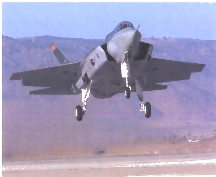
Figure 1.1.3.1 The USA Navy latest generation of fighter aircraft, the Joint Strike Fighter, extensively uses carbon fibre reinforced toughened epoxy resins composites in both primary and secondary structure to reduce weight and improve performance. (Picture courtesy of Boeing Aerospace, Seattle)
