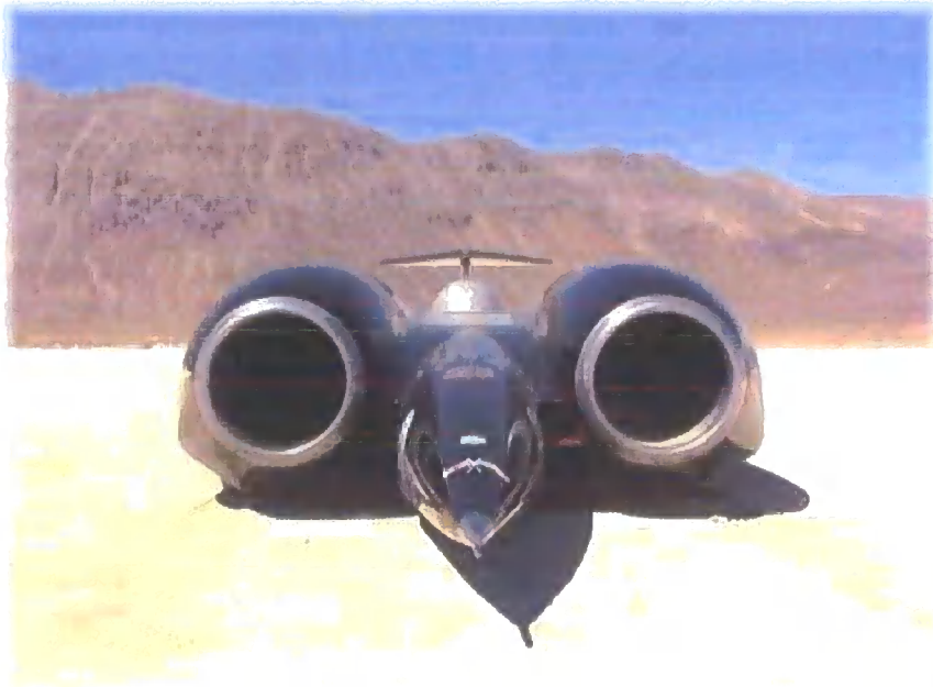
Figure 1.1.1.1 Thrust 2 SSC. This vehicle set the current land speed record of 633.48mph in 1984. Its panel structure was bonded together using a toughened epoxy adhesive (Picture Courtesy of Jeremy Davey of Permabond)
