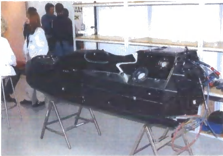
Figure 1.1.3.3 This figure shows a cockpit or so called 'tub' of a formula one car. This is made exclusively from woven carbon fibre reinforced toughened thermosetting epoxy resin
