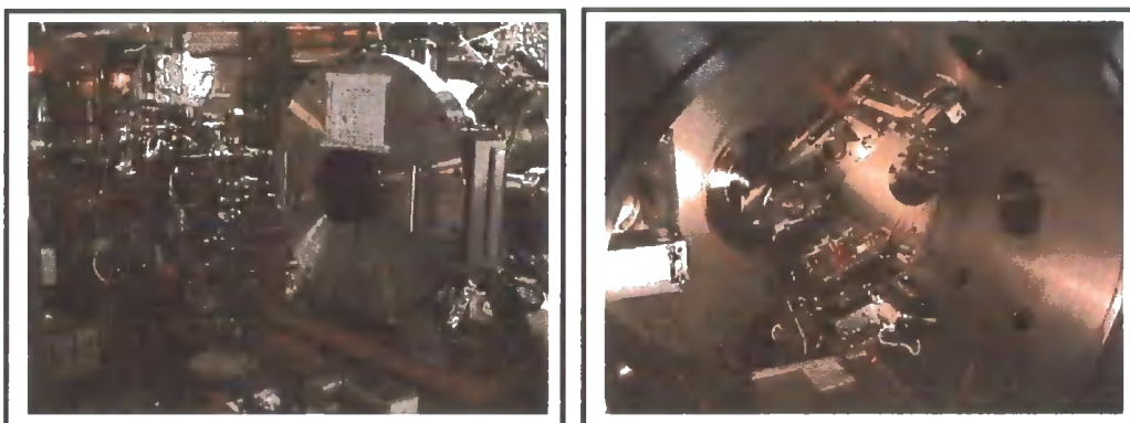
Figure 6.3: In-vacuum 2 circle diffractometer installed on 5U1 at the Daresbury SRS, U.K.
