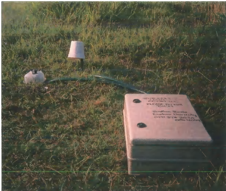
Plate 3.4: Mobile data logger with pyranometer and buried and shaded thermistors on a north-facing slope at Sylvan Dale.
