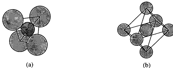
Figure 4.2. Arrangements of oxygen ions surrounding (a) tetrahedral, and (b) octahedral sites. The co-ordination polyhedra are shown.
