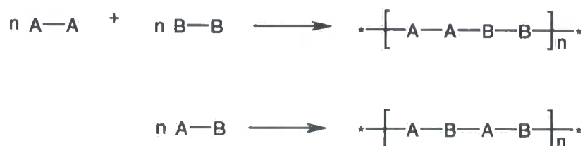
Figure 1.9. Schematic synthesis for linear polymers by step-growth polymerisation.
